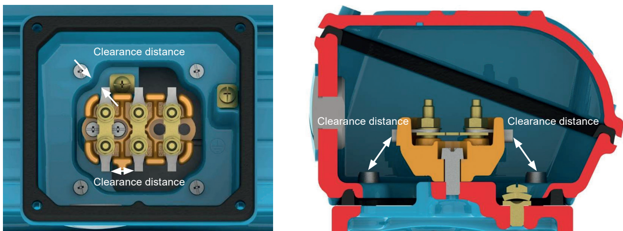
Figure 6.16: Minimum clearance distance (mm) x supply voltage
