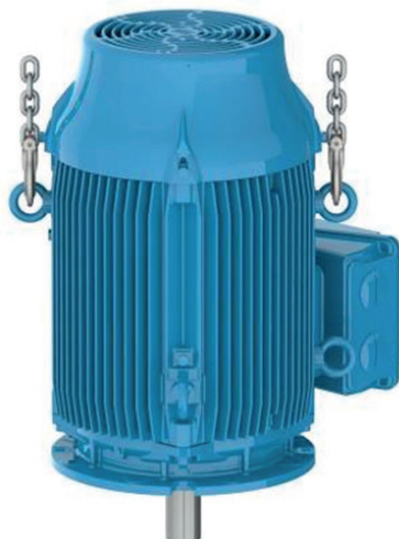
Figure 4.19: Install the first pair of eyebolts
