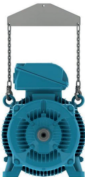
Figure 4.7: Use of a spreader beam for lifting
